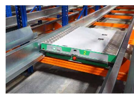
Able to modify the traditional Drive-in Rack to work with the Shutter Cars
